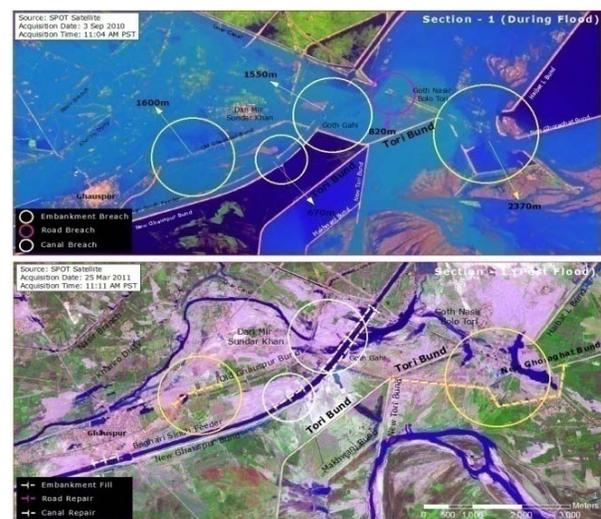
Figure 2.1 Rehabilitation of Tori Breach, Sindh
