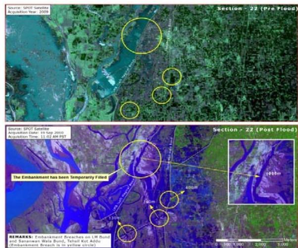
Figure 1.1 LMB Breach near Taunsa Barrage, Punjab
